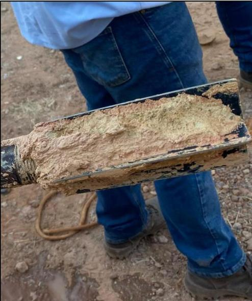
Figure 3.10: Vane with tested soil.
