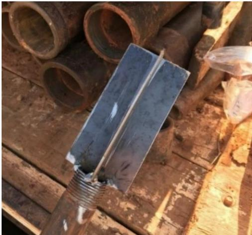
Figure 3.7: The vane used in the tests.
