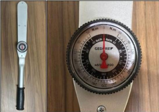
Figure 3.8: The torque wrench used in the VSTs.
