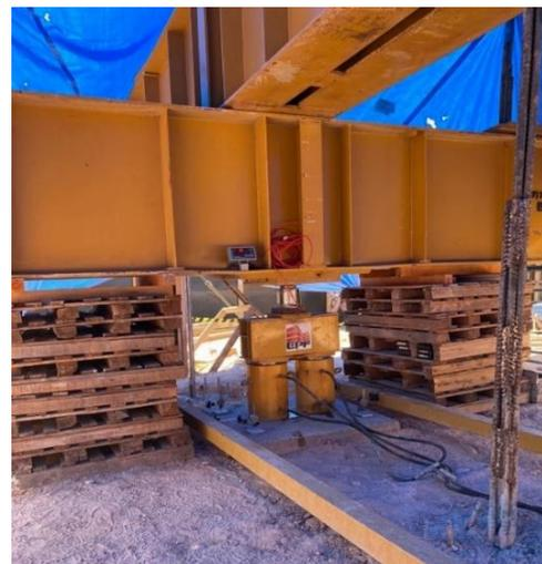
Figure 3.16: Internal view of the load test setup.
