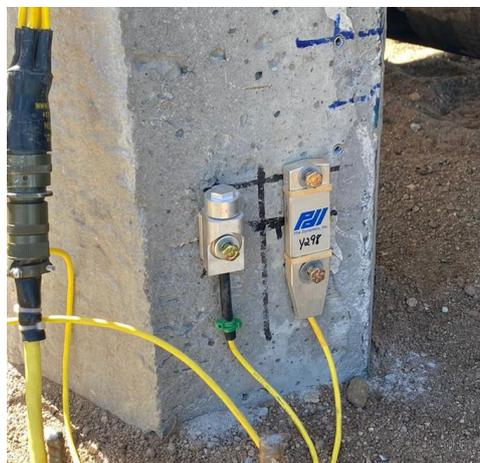
Figure 2.9: Accelerometer (on the left) and strain transducer (on the right).
