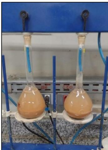
Figure 3.11: Application of vacuum for determination of grain specific gravity.
