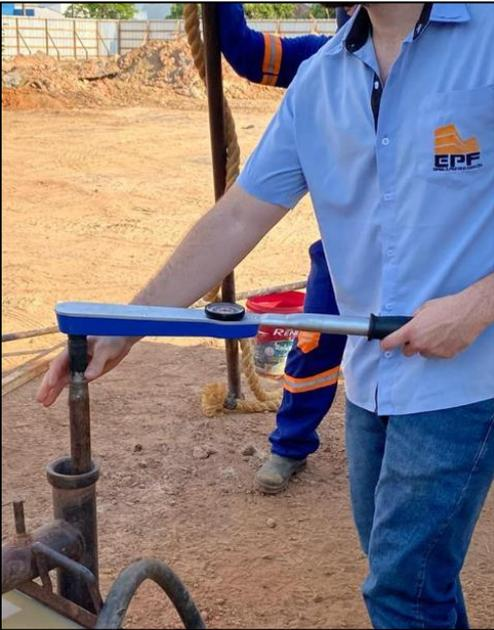
Figure 3.9: Torque application in the VST.
