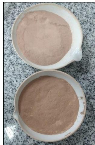
Figure 3.12: Samples used in sieving for determination of Atterberg's limits
