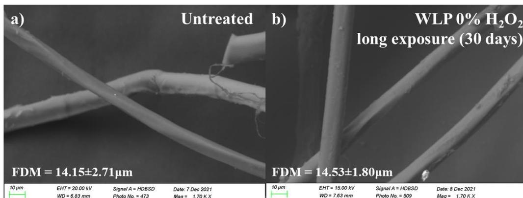
**Figure 47.** Micrographs of fibers after treatment WLP 0% of H<sub>2</sub>O<sub>2</sub> for 30 days.
