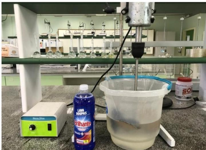
**Figure 19.** Simulating a washing machine
