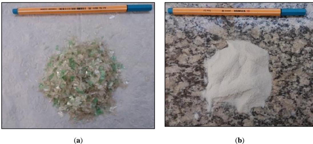
Figure 6: RPET format for use in pavement variants: (a) flake form of 10 mm nominal size; (b) micronized form of 0.42 mm nominal size.
