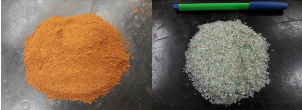
Figure 4: Lateritic soil and RPET used in the study. Extracted from Carvalho et al, (2019).
