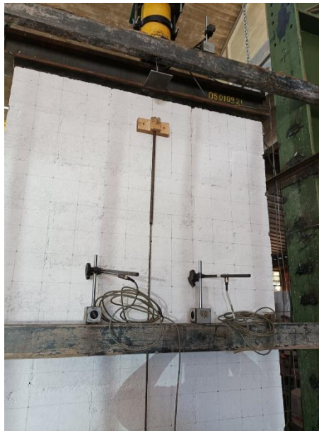
Figure 3.5 - Position of LVDT 1 for the masonry wall W1 test.
