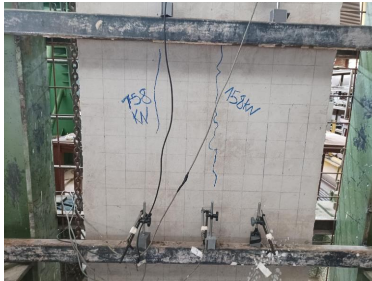
Figure 4. 13 - First cracks visible in panel PA1 test.
