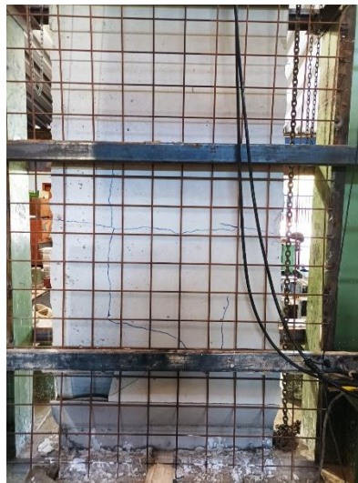
Figure 4. 17 - Cracks in panel PA2 after failure.
