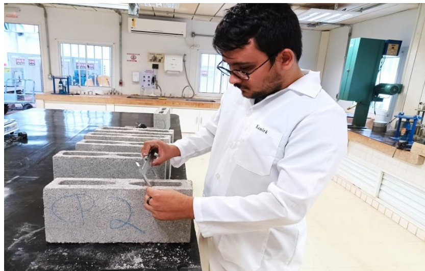
Figure 3. 9 - Measurement of concrete block dimensions.
