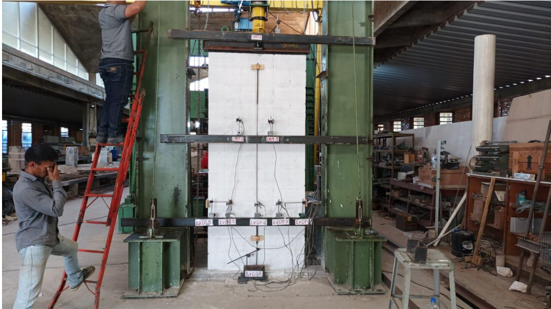
Figure 3.4 - First masonry wall test detail.
