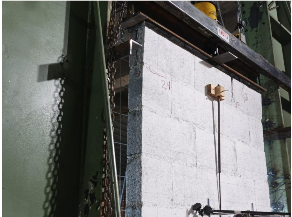
Figure 4. 6 - Crack pattern of wall W1.
