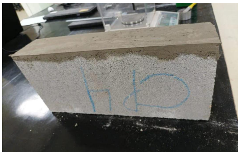
Figure 3. 10 - Regularization layer of cement paste, cast in the hollow concrete blocks for the compressive test.
