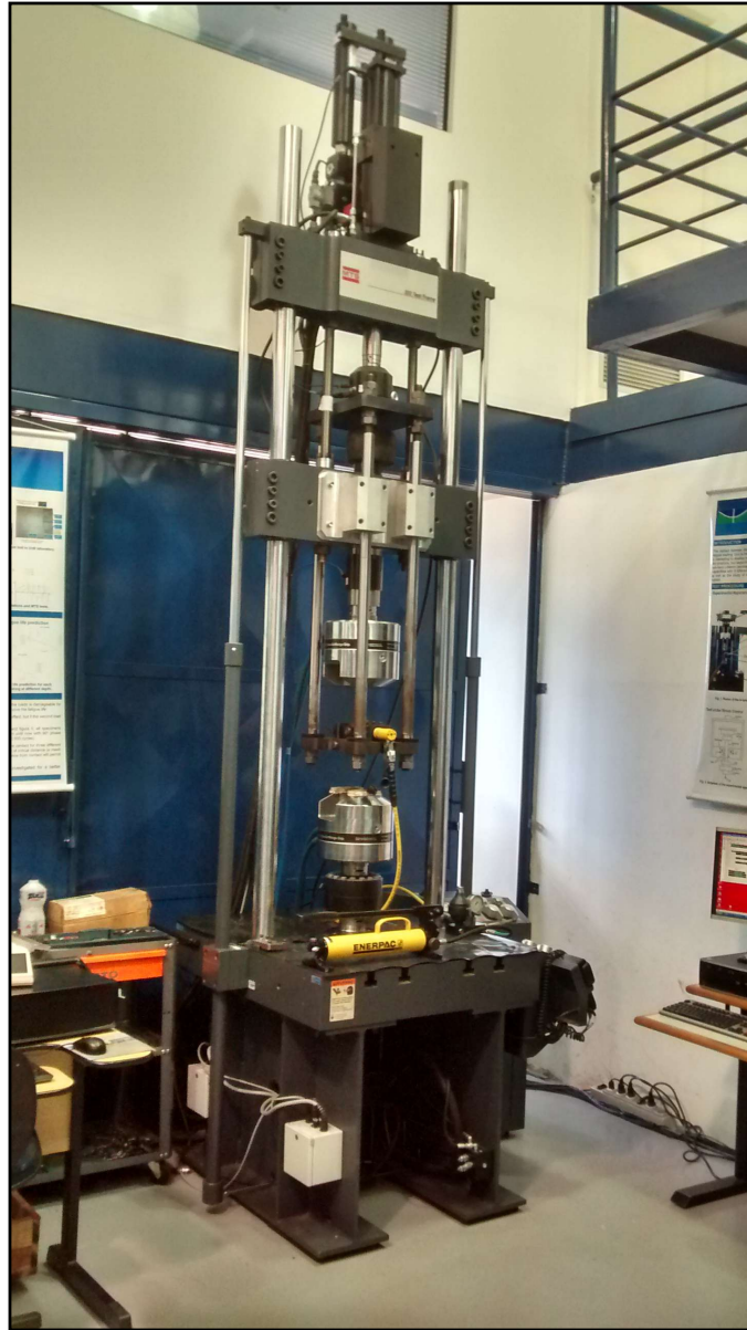
Figure 3.4: Previous version of the UnB's Fretting Fatigue Machine.
