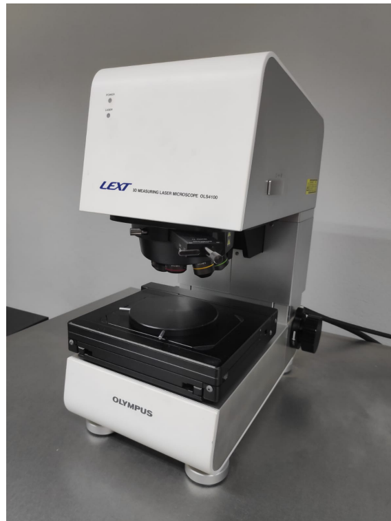
Figure 4.5: Photo of the Olympus LEXT OLS4100 confocal laser microscope.
