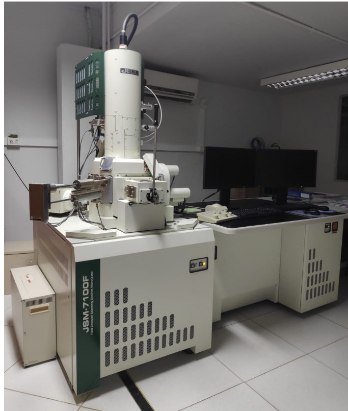
Figure 4.19: Photo of the JEOL JSM-7100F scanning electron microscope.
