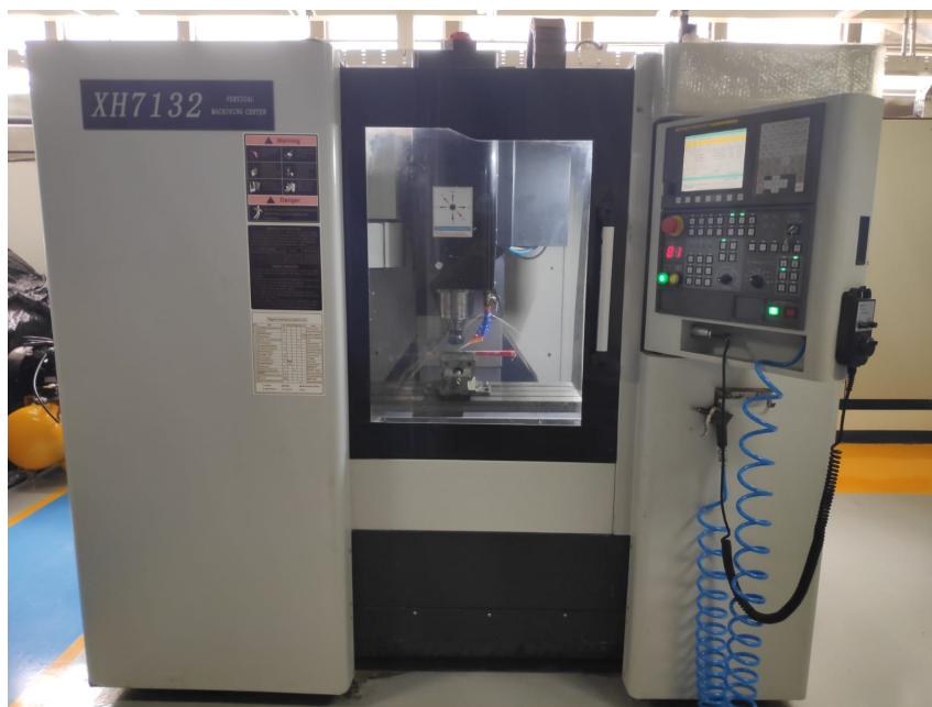
Figure 3.25: Photo of the XH7132 Vertical Machine Center.
