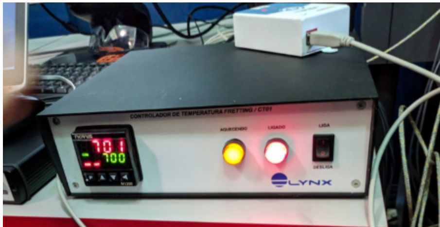
Figure 3.15: Lynx Technology Temperature Controller in operation.
