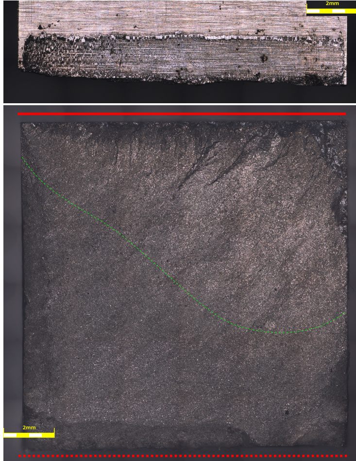
Figure 4.14: Fretting fatigue contact scar and fracture surface of a test with Ti-6Al-4V at RT and constant contact normal load (ff-ti-rt-pc-04).
