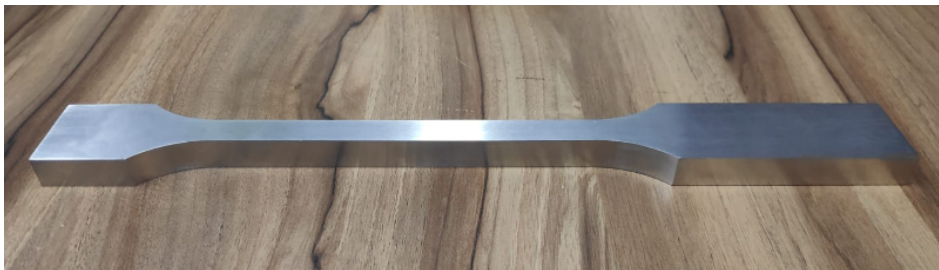
Figure 4.3: Photo and dimensions of the fretting specimen.
