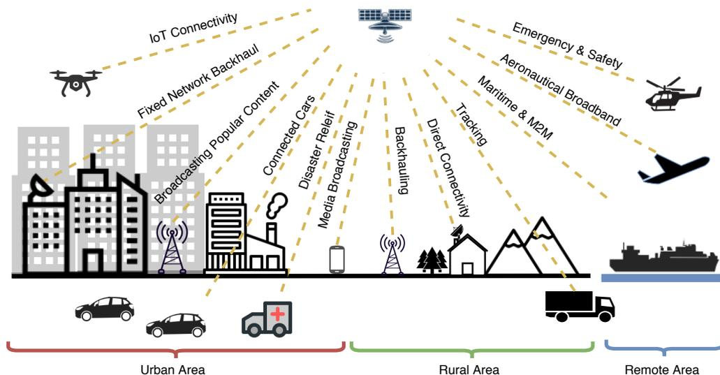
Figure 1 – Diagram describing the role of satellite communications in the 5G communication ecosystem, adapted from [42].
