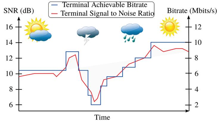
Figure 2 – Relationship between the weather conditions and the maximum bitrate capacity achievable, adapted from [21]
