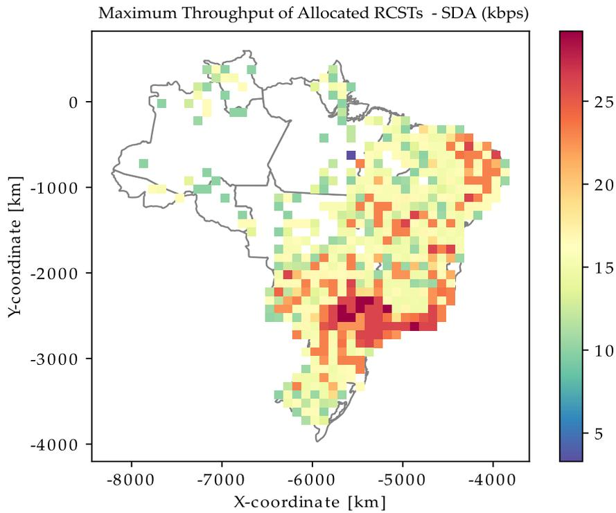
Figure 19 – Heat map of maximum RCST data throughput under the selected coverage area using the SDA algorithm.
