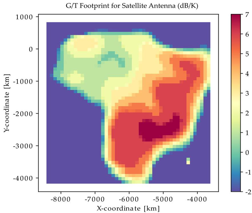
Figure 20 – Heat map of  $G/T$  for a GEO satellite, used as a parameter to obtain spatial information of system performance.
