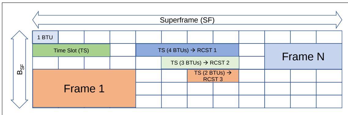
Figure 5 – Diagram illustrating the hierarchy of elements in the DVB-RCS2 SF.
