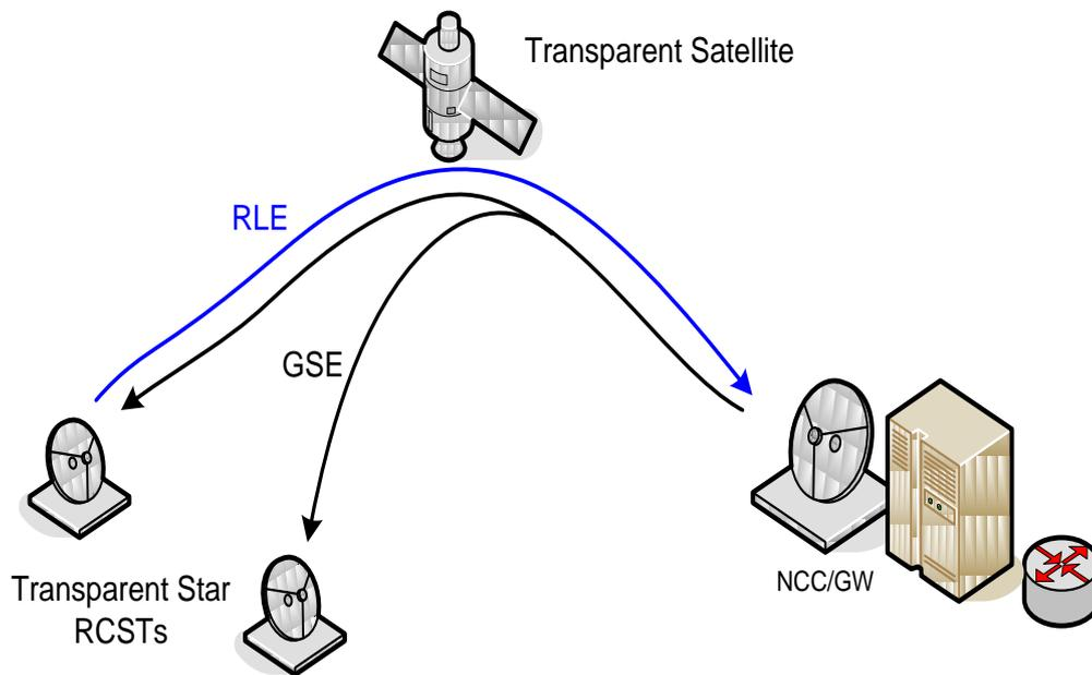
Figure 4 – Star-only topology scenario for communication in DVB systems for Transparent Satellites (adapted from [7]). RLE stands for Return Link Encapsulation and GSE stands for Generic Stream Encapsulation.
