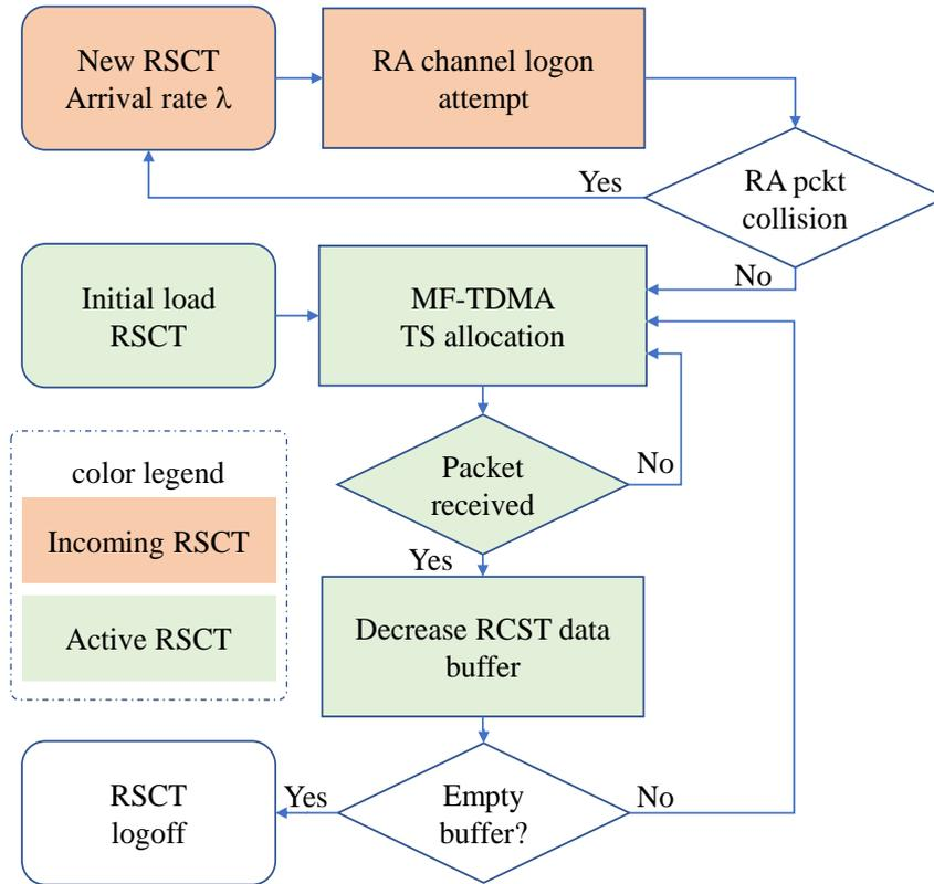
Figure 9 – Terminal lifecycle in the system. Optimization of resources within the RCS-2 MF-TDMA structure is performed at each superframe.
