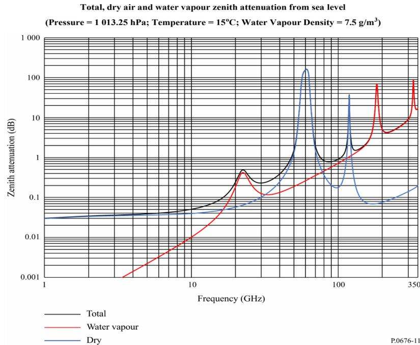
Figure 3 – Relationship between the link’s frequency and the Zenith attenuation by water vapour and dry air, adapted from [44, p. 29]
