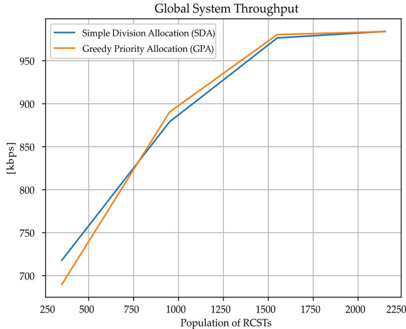
Figure 15 – Global throughput of GPA and SDA allocation algorithms for different load points.
