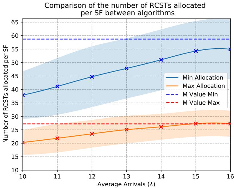
Figure 27 – Average RCSTs allocated per SF comparison between *Max allocation* and *Min Allocation* algorithms and its respective  $m$  value predictions.
