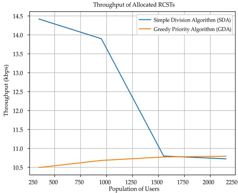
Figure 16 – Average throughput per user of each allocation algorithm for different load points.
