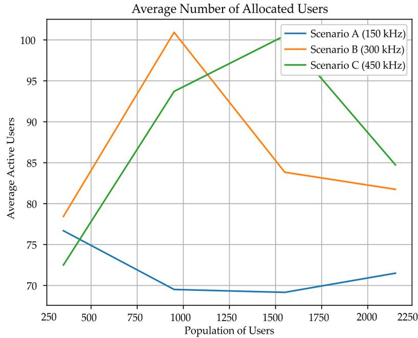
Figure 22 – Average number of active users in the system affected by the collision rates shown in Figure 21.
