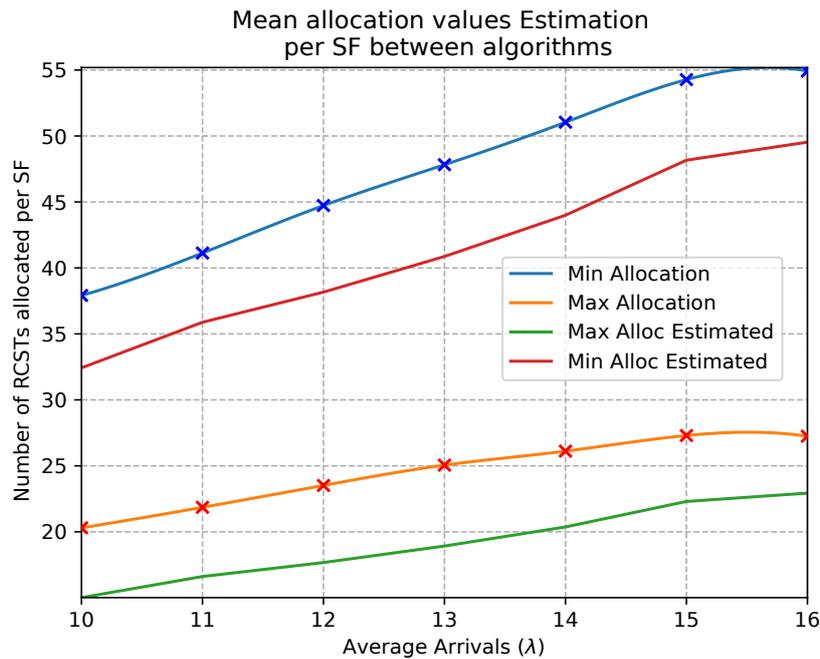
Figure 28 – Comparison between predicted and measured mean allocated RCSTs per SF.
