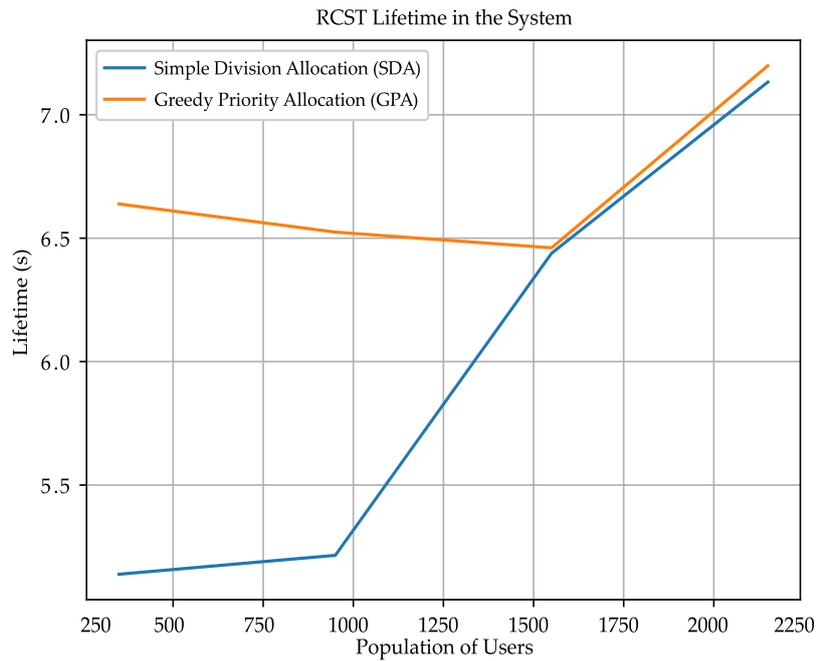
Figure 17 – Average lifetime in seconds of completed users of each allocation algorithm for each load point.
