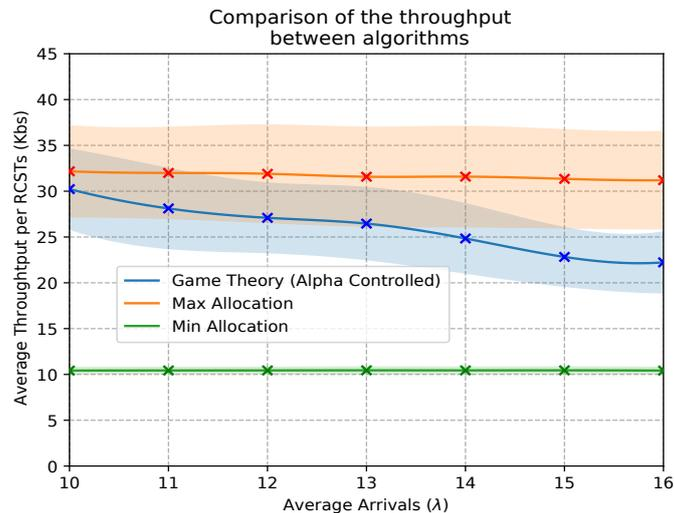
Figure 33 – Comparison between average throughput per SF between resource allocation algorithms.
