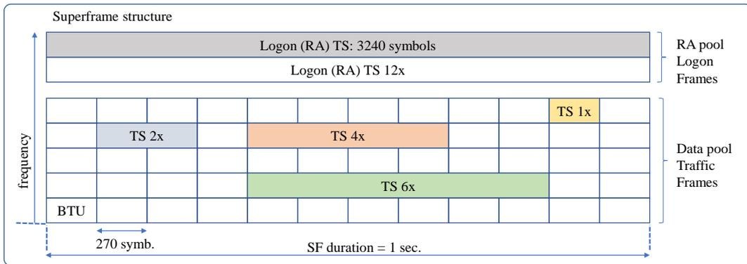
Figure 13 – Organization of the MF-TDMA hierarchy in the simulator (SF, frame, TS and BTU) with two pools of channels: RA for signaling and DA for traffic data. All logon messages use 12 BTUs as a worst case for Waveform 41 in Table 10.4 in [7]. The data BTUs are dynamically allocated, based on current  $E_s/N_0$  and recommended waveforms, both obtained from link level simulations.
