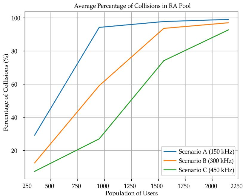
Figure 21 – Average percentage of collisions in the RA frames for different proportions of RA and DA pools. In all cases, the system has the same total bandwidth.
