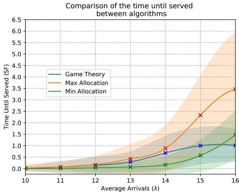
Figure 29 – Measured time until served for different resource allocation algorithms.
