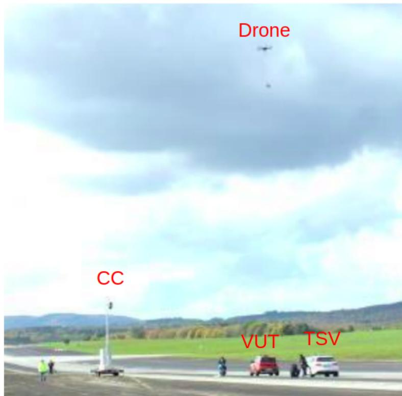
Figure 1.2: Modelling of the test track scenario using drones, CC designates the command central, VUT is the vehicle under test and TSV is a traffic simulation vehicle.
