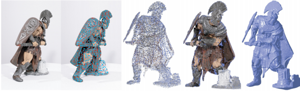
Figure 3.12: An overall approach of a patch-based MVS model reconstruction. From left to right: A sample input image; detected features; reconstructed patches after the initial matching; final patches after expansion and filtering; and the mesh model [11].
