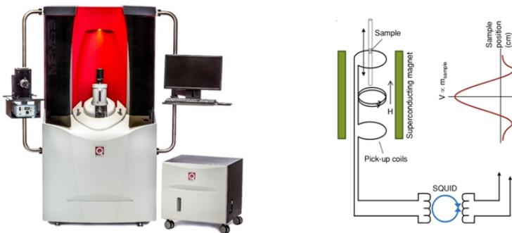
**Fig. 3.3** (Left) MPMS magnetometer of the Magnetic Characterization Laboratory of the Institute of Physics at the University of Brasilia and, (right) Schematics of the SQUID-based measurement system [21].
