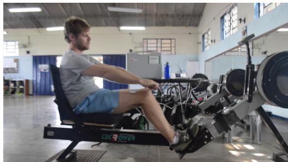
Figure 6.1: Ergometer for rowing. We used the measures of this ergometer to develop the additional parts of the FES rowing model.
