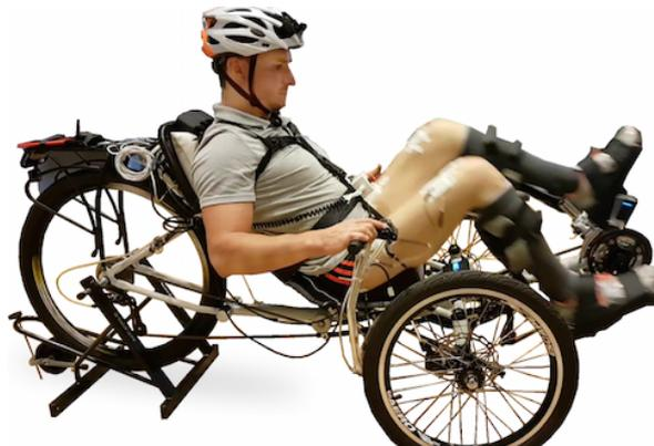
Figure 5.1: The adapted tadpole trike (HP3, Brazil). We used the measures of this tricycle to develop the additional parts of the FES cycling model (Bó et al., 2017).
