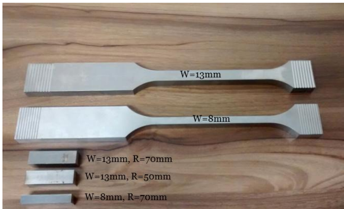
Figure 3-9: Photograph of fretting fatigue specimens and pads.
