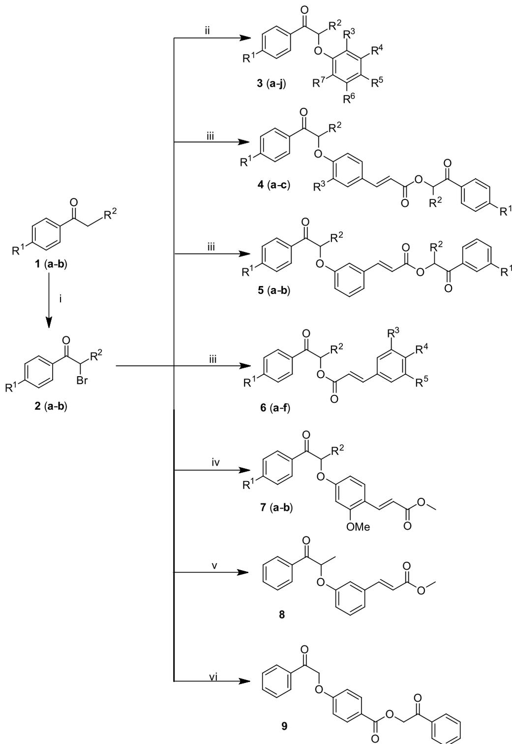
**Scheme 1.** Synthesis of 8,4'-oxyneolignan analogues. Reagents and conditions: (i) Br<sub>2</sub>, CHCl<sub>3</sub> r.t. 2 h; (ii) ArOH, K<sub>2</sub>CO<sub>3</sub>, butanone or MeCN, 80 °C, 12 h; (iii) cinnamic acids, K<sub>2</sub>CO<sub>3</sub>, butanone or MeCN, 80 °C; (iv) methyl ferulate, butanone or MeCN, 80 °C, 12 h; (v) methyl 3-hydroxycinnamate, K<sub>2</sub>CO<sub>3</sub>, butanone or MeCN, 80 °C; (vi) 4-hydroxy-benzoic acid, K<sub>2</sub>CO<sub>3</sub>, butanone, 80 °C.
