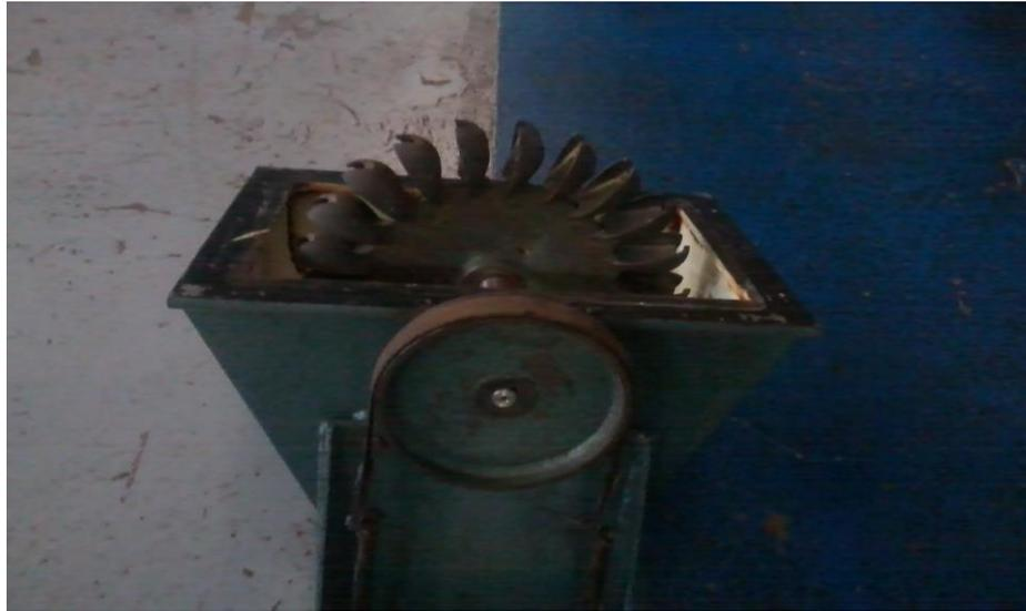
Figura 4. Turbina Pelton
