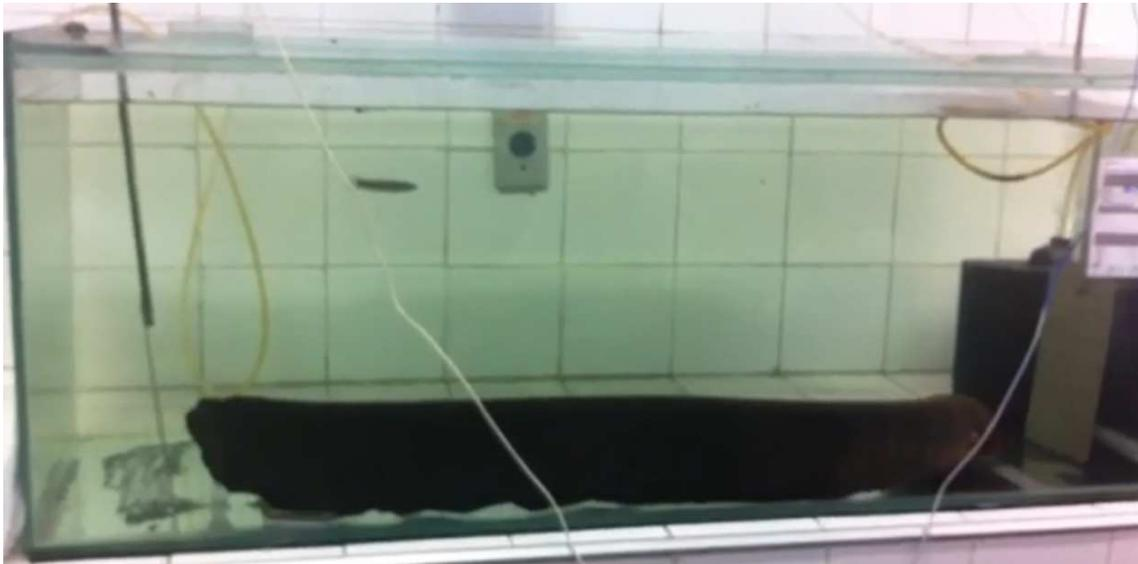
Figure 3.20: Real experiment carried out in LFCE-INPA, wherein the electrodes are metal plaques with a resistance of  $4 \Omega$  each. This photo was made while the electric eel swam in order to look for the prey, which is the little fish in the above part of the aquarium, near to the surface.
