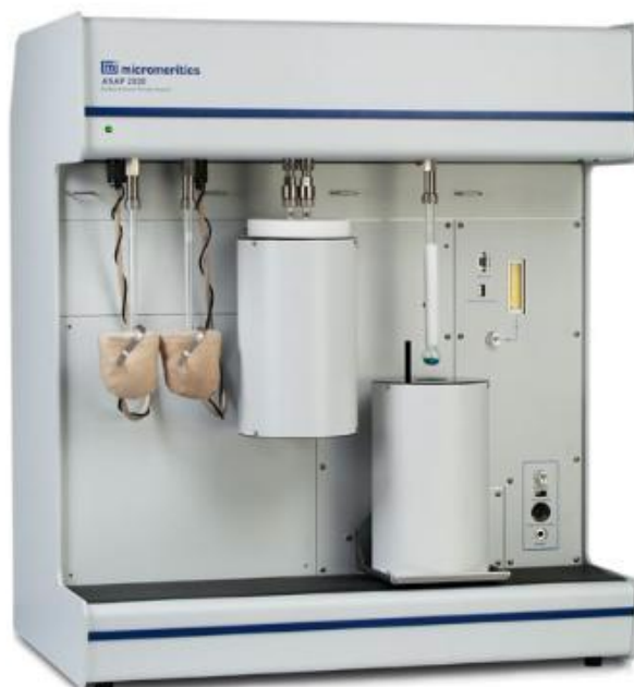
Figura 18. ASAP 2020 (Accelerated Surface Area and Porosimetry System), Micromeritics. 47
