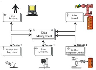
Figure 3. Parallel multi-sensor system "ParMan", indicating employed transputer nodes.
