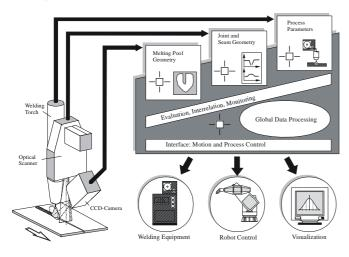
Figure 1. Set up and functional main units of the multi-sensor welding system.
