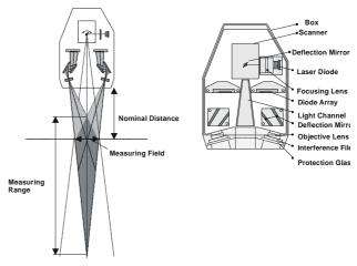
Figure 4. Joint welding sensor set up (detailed view).
