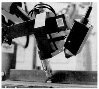
Figure 4. Joint welding sensor set up (real view).
